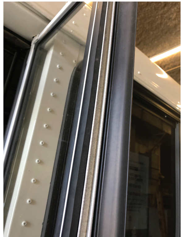
ME110 sensing edge + ME110-C3 mounting channel installed on operating rear passenger door
